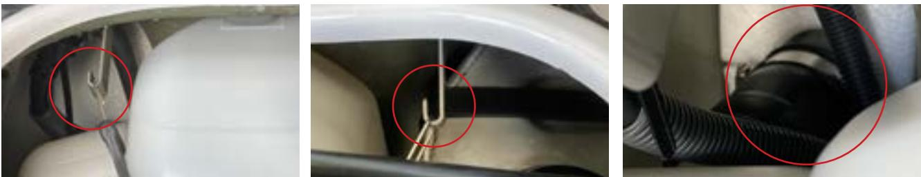
4. Install WORX Silicone hose to outlet and waterbox and secure with OEM clamps. DO NOT overtighten clamps.
