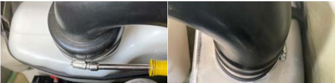
3. Remove sound suppression baffle straps and elbow hose connected to thru-hull fitting. Discard baffle. Retain OEM clamp.
