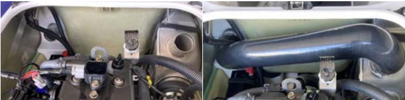
5. Check ski for tools etc. Re-connect battery and run on flush hose to check for leaks.
